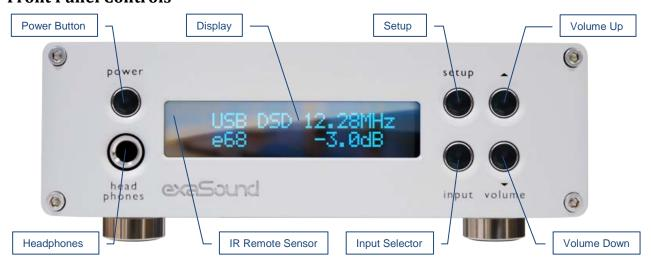
**Headphones** accepts a standard 1/4-inch stereo single-ended phone plug. Use a suitable adapter for headphones equipped with a different plug.
